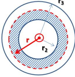
$$\oint \vec{B}_O \cdot d\vec{l} = \mu_0 (I - I_{in \ contur}), \quad I_{in \ contur} = j_{camasa} (\pi r^2 - \pi r_2^2), \quad j_{camasa} = \frac{I}{\pi (r_3^2 - r_2^2)},$$
