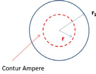
$$\oint \vec{B}_M \cdot d\vec{l} = \mu_0 I_r, \quad B_M 2\pi r = \mu_0 I_r, \quad I_r = j\pi r^2, \quad j = \frac{I}{\pi r_1^2}, \quad B_M 2\pi r = \mu_0 \frac{I}{\pi r_1^2} \pi r^2, \quad B_M = \frac{\mu_0 I}{2\pi r_1^2} r$$
