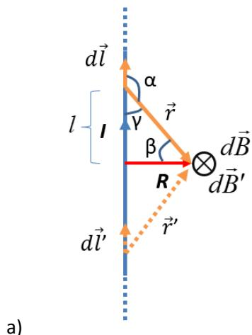
$$d\vec{B} = \frac{\mu_0}{4\pi} I \frac{dl \times \vec{r}}{r^3}, \quad dB = \frac{\mu_0}{4\pi} I \frac{dl}{r^3} \sin \alpha, \quad \alpha = \beta + \frac{\pi}{2}, \quad \sin \alpha = \sin \left( \beta + \frac{\pi}{2} \right) = \cos \beta$$
